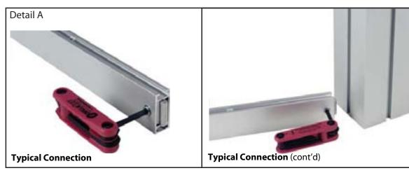
Most horizontal extrusion connections have a patented expandable lock. This lock inserts into the groove of an opposing extrusion. Tightening the lock with the Hex Key Tool expands the lock and creates a strong positive connection.
